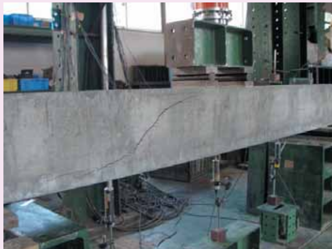
Diagonal shear failure at high strength RC beam
