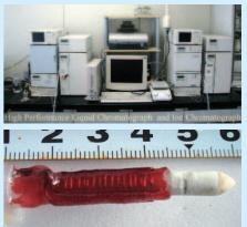
Small Time Domain Reflectometry-Tensiometer coil probe
